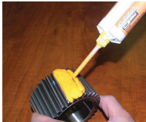
Shown Above: Quick Dispense internal casting (left) and external casting (right) using the new Flexbar Repo-Mix II Dispensing Gun System.
